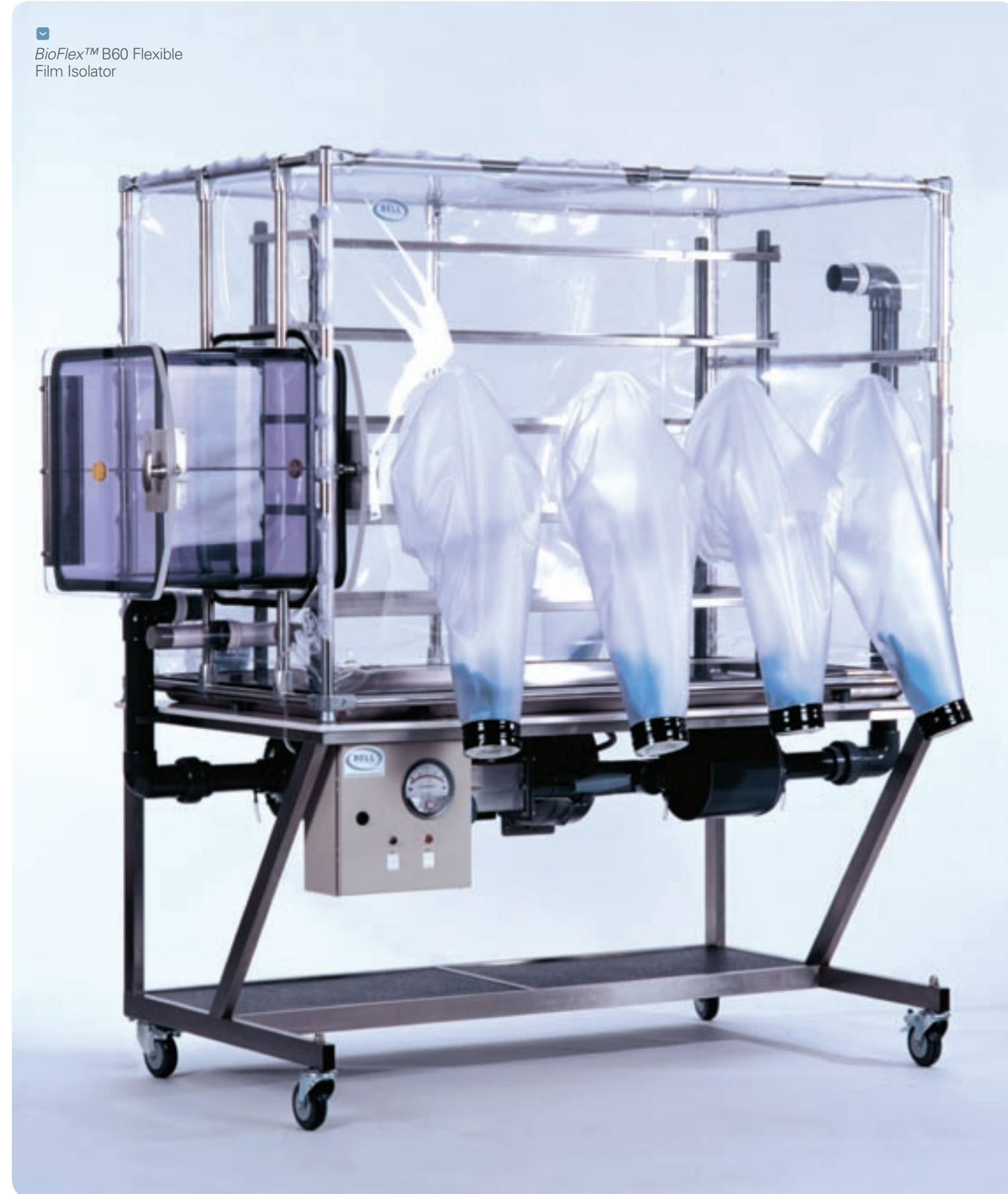
▶ HEPA Filtered Ventilation System with negative or positive pressure operation, changeable in seconds
