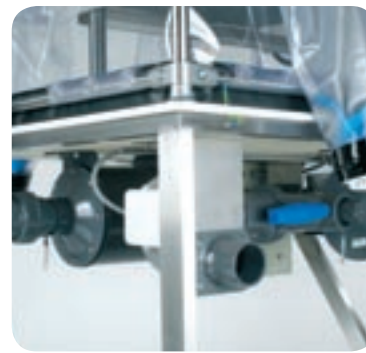
▶ HEPA Filtered Ventilation System with negative or positive pressure operation, changeable in seconds
